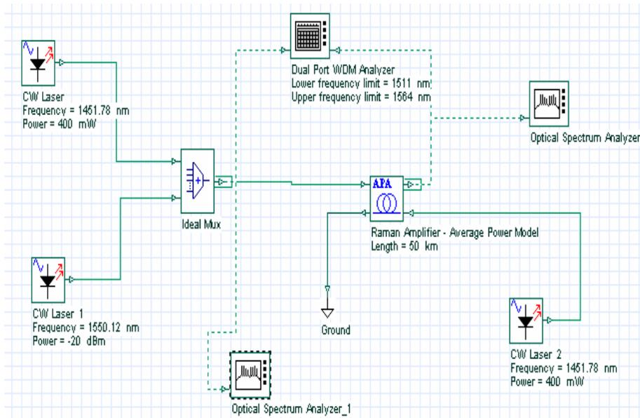
Fig. (2): the simulation layout, bidirectional pumping
